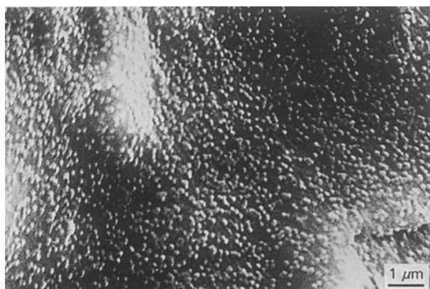
Figure 5 SEM micrograph of the anorthite glass heat treated at 1000 °C for 2 h ( \phi = 10 °C per min), furnace cooled, and etched at 25 °C with 1% HF for 20 sec. Prior to the heat-treatment, the sample was nucleated at 880 °C for 2 h and a \phi = 10 °C per min.
